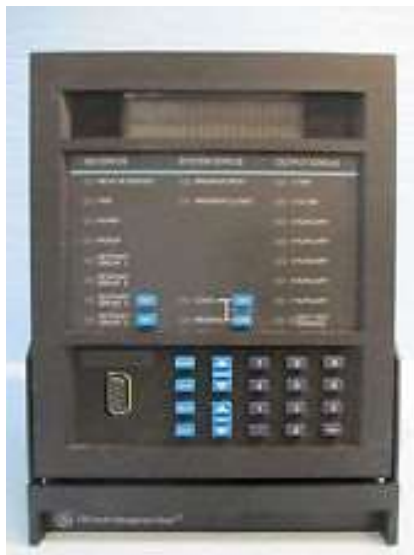
GE Multilin Relay 469 Simulator
