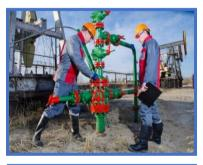
Christmas trees are used on both sub-surface and subsea wells. It is common to identify the type of tree as either "subsea tree" or "sub-surface tree". Each of these classifications has a number of variations. The primary function of a tree is to control the flow, usually oil or gas, out of the well. A tree may also be used to control the injection of gas or water into a non-producing well in order to enhance production rates of oil from other wells.
